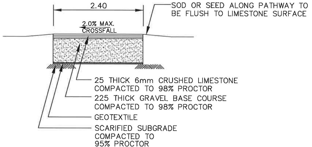
TYPICAL CRUSHED LIMESTONE PATHWAY
