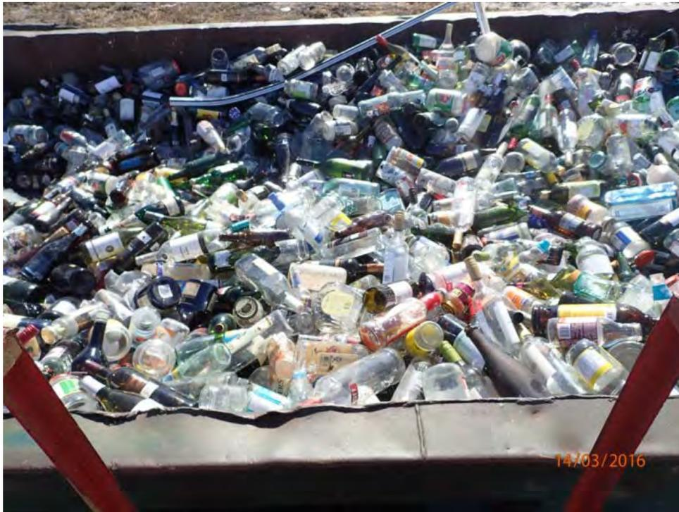
*b) Glass recycling container with some visible non-glass material*
