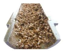
Pipe clogged with zebra mussels, resulting in 40% water flow reduction
