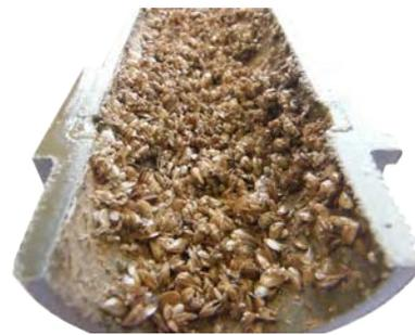
Pipe clogged with zebra mussels, resulting in 40% water flow reduction
