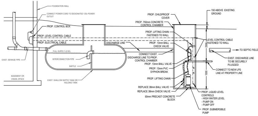
1 TYPICAL LPS SERVICE CONNECTION (TYPE A - EXISTING HOLDING TANK WITH PUMP OUT CONTROL CHAMBER ADDED)
