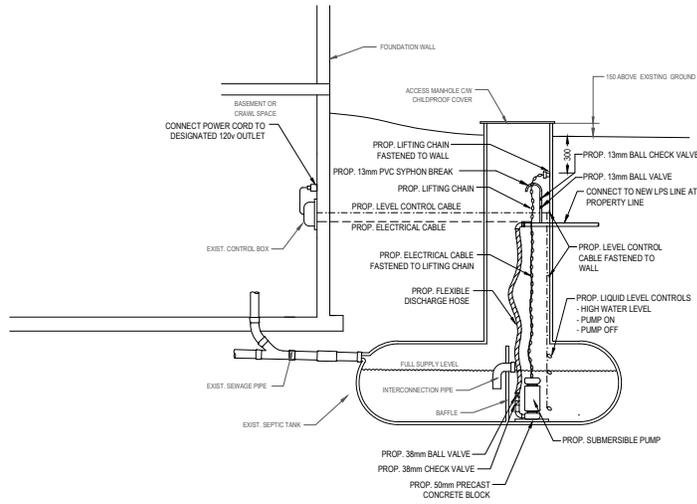
2 TYPICAL LPS SERVICE CONNECTION (TYPE B - EXISTING SEPTIC TANK)
